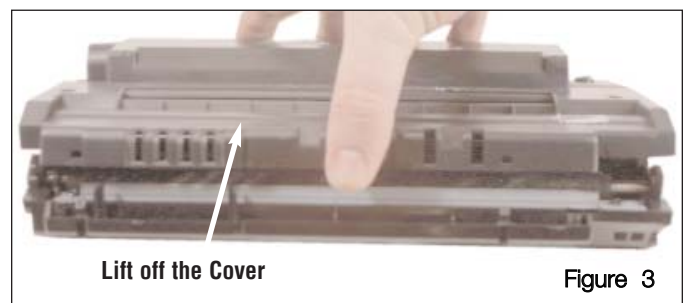
Lift off the top of the cartridge.
