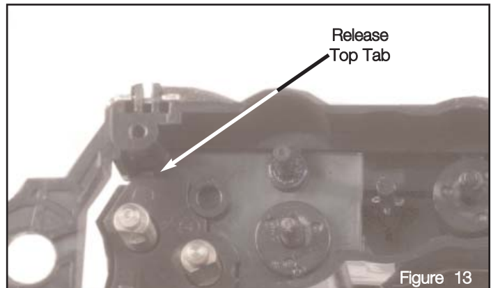
Release the top tab of the Developer Roller Plate.
