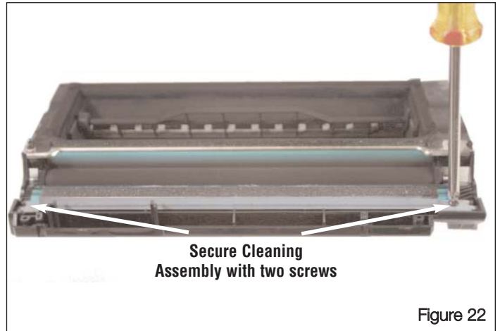
Install the Cleaning Assembly.
