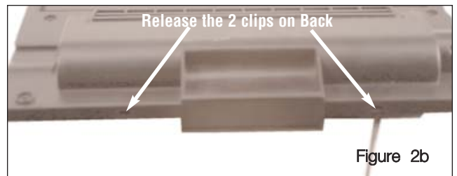
Release the four clips that secure the two sections together
